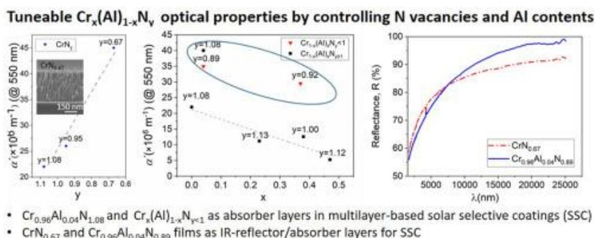
In order to explore the potentialities of  $\text{Cr}_{1-x}(\text{Al})_x\text{N}_y$  materials in multilayer-based solar selective coatings (SSC) for high temperature applications ( $T > 500^\circ\text{C}$ ), the optical behavior of  $\text{Cr}_{1-x}(\text{Al})_x\text{N}_y$  films is studied in this work. Two sets of layers ( $\text{CrN}_y$  and  $\text{Cr}_{1-x}\text{Al}_x\text{N}_y$ ) were prepared by direct current (DC) and high-power impulse magnetron sputtering (HiPIMS) technology. The
