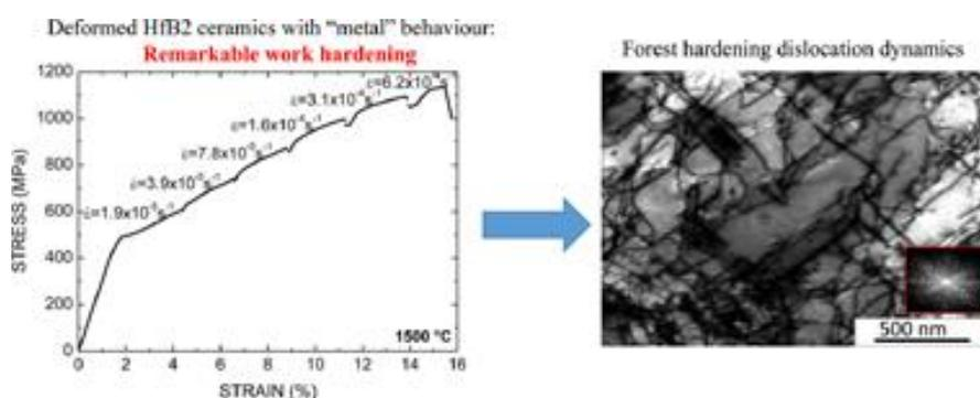
Hafnium diboride ( $\text{HfB}_2$ ) is a highly refractory (melting above 3000 °C) ceramic with many potential applications at high temperatures. To enable its use at temperature for extended periods its high-temperature plasticity must be known. This paper examines the mechanical response at temperatures between 900 °C and 2000 °C in air and in a reducing atmosphere, interpreting the data in the frame of classical models for the plasticity of compact-packed metals
