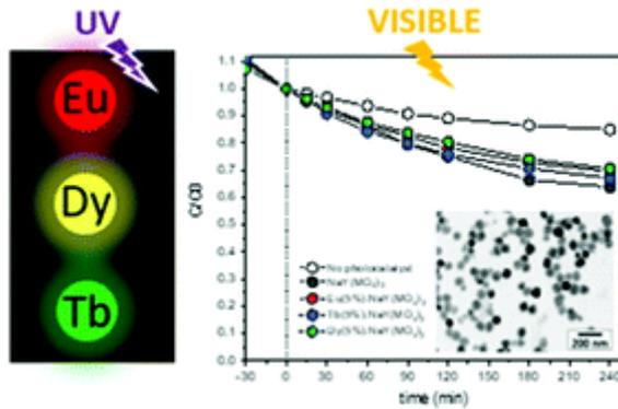
The effects of the cations doping level on the luminescent properties are analyzed in terms of emission intensities and luminescent lifetime, to find the optimum phosphors. Finally, the performance of these nanophosphors and that of the undoped system for the photocatalytic degradation of rhodamine B, used as a model compound, is also analyzed.
