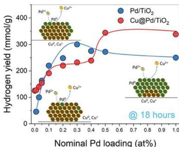
Different Cu@Pd-TiO<sub>2</sub> systems have been prepared by a two-step synthesis to obtain a bimetallic co-catalyst for the H<sub>2</sub> photoreforming reaction. We find that the tailored deposition of Pd covering the Cu nanoclusters by a galvanic replacement process results in the formation of a
