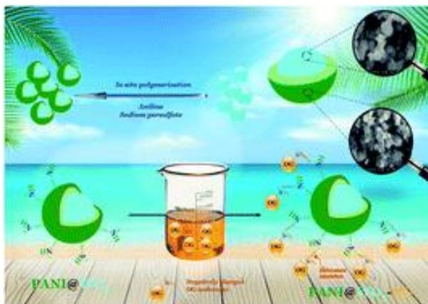
adsorption process occurred spontaneously and endothermically. Importantly, PANI@WO<sub>3</sub> still exhibited an excellent adsorption capability after four regeneration cycles, indicating the potential reusability of the PANI@WO<sub>3</sub> composite. These results indicate that the as prepared PANI@WO<sub>3</sub> composite could be employed as an efficient adsorbent and was much better than the parent material adsorption of OG dye.
