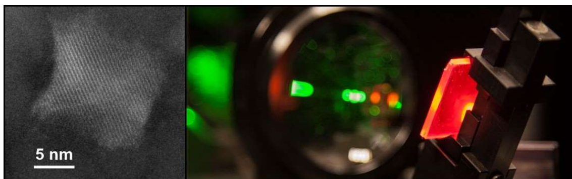
Illustrative images of (left) a perovskite nanocrystal synthesized in the multifunctional Optical Materials group and (right) a photoluminescence material while being characterized in our labs.
